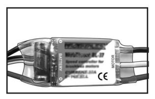
□Battery:5 cells -18.5v 4000 - 5000mah Li -Po
