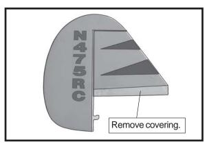
□ 3) Slide the vertical stabilizer back in place. Using a triangle, check to ensure that the vertical stabilizer is aligned 90° to the horizontal stabilizer.
