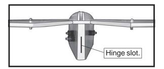
$\Box$  2) Glue the vertical fin in place using as same as techniques used to installing the horizontal fin.
