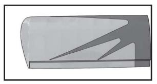
Note: <u>Work the aileron up and down several</u> <u>times to "work in" the hinges and check</u> <u>for proper movement.</u>
