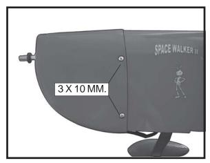
Secure the cowl with the screw provide with hardware.
