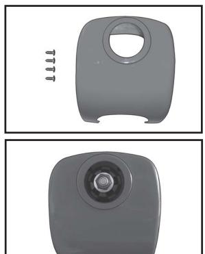
Slide the fiberglass cowl over the engine and line up the back edge of the cowl with the marks you made on the fuselage then trim and cut.
