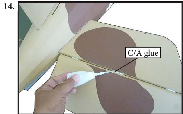
Gently pull on the fixed and moving surface to make sure the hinges are glued securely. If not, reapply thin CA to any hinges that are found loose.
