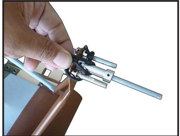
Wrap the cord back around the rear axle support. Continue to wrap the shock cord six times around all the supports for the landing gear.
