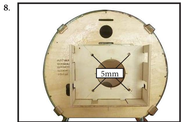
Attach the motor mount to the front of the electric motor box using four 5mm blind nut, four M5x20mm hex head bolts to secure the motor. Please see picture shown.
