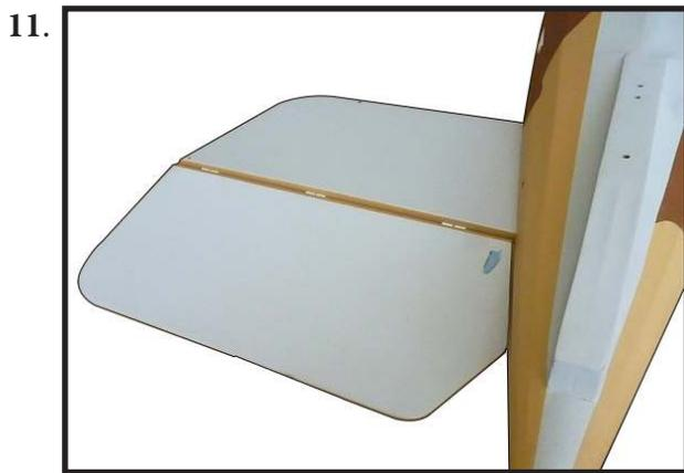
Check the fit of both elevators at this time. Once checked, remove the elevators.
