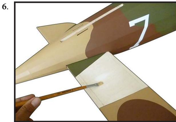
Carefully turn the model over and apply epoxy to the exposed wood on the bottom of the stabilizer. Slide the stabilizer back into position.
