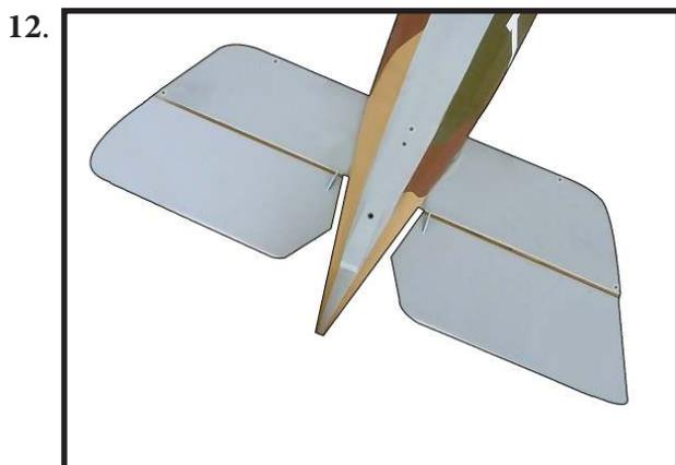
Fit the elevators back into position. Remove the T-pins and slide the elevators tightly against the stabilizer. Use a paper towel and isopropyl alcohol to remove any excess epoxy before it begins to cure.
