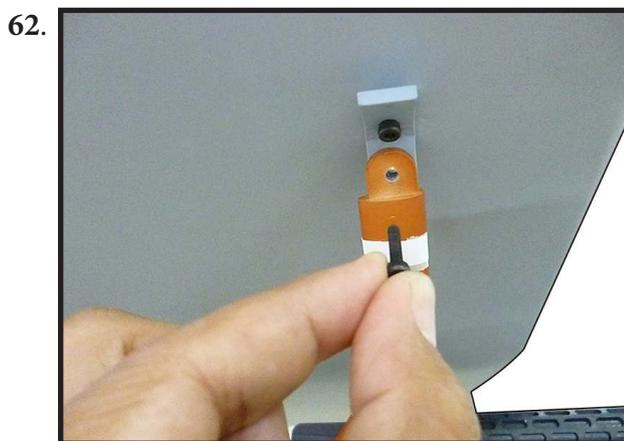
Take the number 6 strut in the middle and attach it to the fuselage. connect from 2 to 5.
