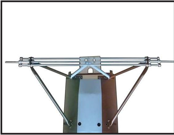
Tie the shock cord to the rear axle support. Leave 1/2-inch (13mm) of shock cord outside the knot so the opposite end of the shock cord can be secure to it.
