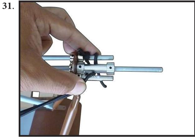
Use a tie wrap to secure the shock cord ends together. Use hemostats to hold the shock cord while installing the tie wrap.
