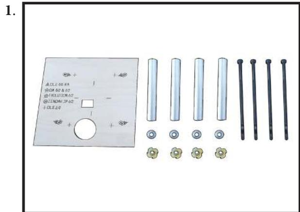
Locate the engine mounting in position on the firewall. Use a 2.5mm drill bit to drill the holes necessary to mount your particular motor choice.
