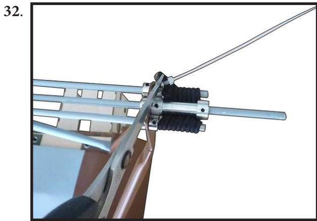
Cut the excess of the tie wrap so the landing gear wing cover can be installed. When the shock cord is installed, it will fit inside the landing gear wing and will not interfere with the installation of the cover. Tighten all the hardware associated with the landing gear at this time.
