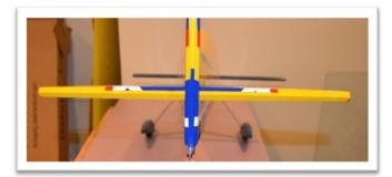
Position the stabilizer perpendicular to the fuselage and parallel to the main wing tube. Measure the distance between the canopy latch and the corners of the horizontal stabilizer. Adjust the stabilizer until the measurements on both sides are equal. Continue checking the stabilizer to ensure it is still centered side to side as described above. Extra time spent here will go a long way to improve the flight characteristics of your airplane.
