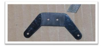
Tests fit the control horn to the slot. Use a file to modify the slot as needed. Center it side to side and align the holes with the hinge line. The control horn should be symmetrical about the hinge line.
