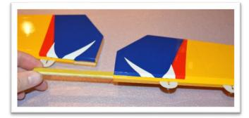
Install a control horn in the elevator using the same procedure used when assembling the ailerons. <u>Make</u> sure you are working with the left elevator half.
