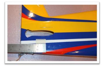
Slid the horizontal stabilizer through the fuselage pushing it all the way forward. Center it side to side using a ruler or tape measure.
