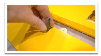
The control horn should go all the way in until the shoulder contacts the aileron. The linkage hole in the control horn should be aligned with the hinge centerline.
