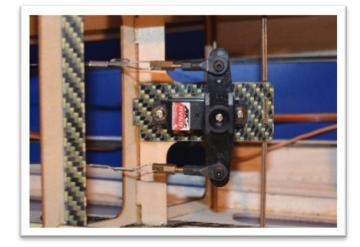
Thread on 2 crush sleeves and the brass cable eye.
