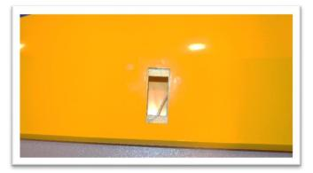
Gently pull off the servo wire installation string and temporarily secure it out of the way. Do not pull it out of the wing. (If there is glue left behind scrape it off so the wood mounting surface is flat.)
