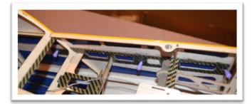
Cut open the pocket just after the second small hole. This is where the aileron servo wire will enter the fuselage.
