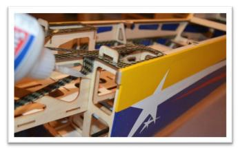
Locate the mounting holes for the wing. Use an iron to seal the covering around the edges of the pocket before trimming. There will be 2 holes for wing alignment pins, 1 hole for the wing bolt, 1 slot for the servo lead, and 1 large hole for the wing tube. Measuring from the front edge of the firewall the holes can be found at 3'', 5 7/8'', 7  $\frac{1}{2}$  %''. You can also locate the holes by pocking a pin through the covering from the inside out.
