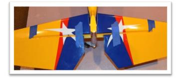
After the epoxy has had plenty of time to cure remove all the masking tape.
