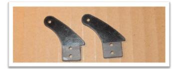
Test fit the control horn in the slot. Trim or file the slot as needed to achieve a snug fit. (Be careful you don't poke through the other side of the aileron.)
