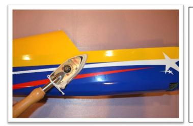
At 200-220°F (93-104°C) the adhesive on UltraCote<sup>®</sup> becomes active allowing the covering to be attached to the model. While 220° will fully bond the covering to the model it is well below the temperature that causes UltraCote<sup>®</sup> to shrink.
