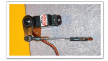
Check the length of the assembly to the servo arm with the aileron level with the wing. When the correct length of the assembly is found, connect the ball link to the servo arm. (Always adjust the connecting rod length with the servo powered up and centered.)
