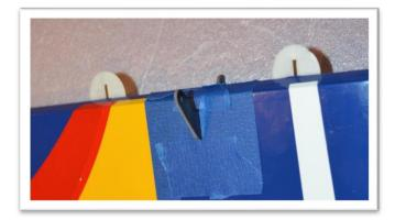
Use 30 minute epoxy to glue the control horns in place. Center the control horn, peal the masking tape away, and clean up with alcohol.
