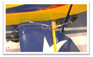
Remove the tape and adjust the cable lengths to center the rudder by turning the cable eyes into the ball links.
