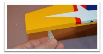
Test fit the elevator joiner plate to the opposite elevator half. Ensure the elevator halves are not twisted. Hold one half of the elevator in position and check the alignment of the other side. Check the gaps at the ends of the stabilizer. Adjust the slot in the elevator or file the edges of the jointer plate as needed to achieve a good fit.
