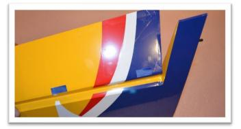
Start with the hinge near the wing tip. Flex the aileron slightly and apply a few drops of thin CA glue to one side. Flex the aileron to its maximum position and return to center. Then glue the opposite side.
