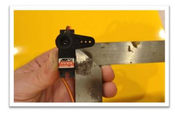
You may use a standard size servo or a mico size with an adapter plate shown below.
