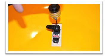
Assemble a ball link to each end of a connecting rod. Use a socket head screw, a flat washer and a nylon lock nut to connect a ball link to the servo control horn. (The brass ball in the link is offset. The larger reveal side should be against the control horn and servo arm shown below.)
