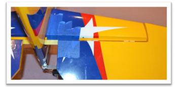
Put the right elevator half in position on the horizontal stabilizer.
