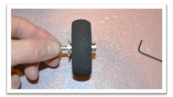
Insert the wheel and axel into the wheel pant, then into landing gear. Align the wheel pant indentation with the landing gear. Add a nylon lock nut and tighten.
