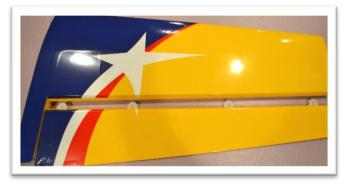
The wings are already slotted for the hinges. Use a covering iron to secure the covering along the edge of the wings. Look at the wing hinge slots closely. Make sure the covering will not interfere when gluing the hinges. Cut away any covering that covers the hinge slot.
