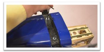
The filler block can be held in position with strips of covering material, packing tape, or it can be held in position with hook and loop material as described below.
