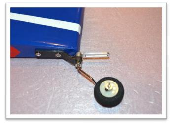
The third screw is used to secure the tiller arm to the rudder after it's installed. Do not fully tighten the tiller arm screw. The slot in the tiller arm allows the rudder to move freely.
