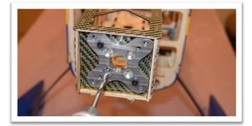
Remove the motor mount and enlarge the holes to 5/16". ( A little CA glue and a file will help clean up the carbon fiber strands and hole shape.)
