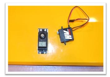
Fit the adapter plate into the servo pocket if you are using the micro size servo. You may need to sand the edges slightly to fit it in. The front corner of the servo pocket should be tilted away from the aileron control horn as shown.
