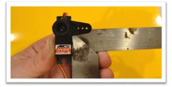
Attach an 18" servo extension onto the elevator servo lead and use a safety clip to secure the connection.
