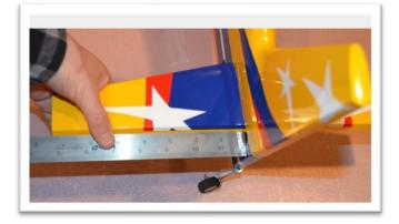
Install and center the main wing tube. Look at the plane from the back forward to make sure that the horizontal stabilizer is parallel with the wing tube. Notice that the horizontal stabilizer is tapered which may obscure the actual alignment. If the stabilizer is not aligned use shims or sand inside the pocket until it's parallel.
