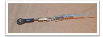
Assemble 2 ball links and cable eyes to the rudder control horn using 2mm screws, a washer, and lock nut.
