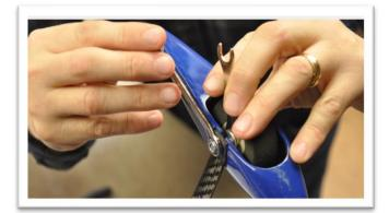
Install the tailwheel using 2 of the 3 wood screws. Position the joint of the tail wheel assembly directly over the rudder hinge line and mark the position of the screws. Turn the screws into the fuselage and rudder. Remove the screws, add a drop of thin CA glue to each hole to strengthen the wood, and reinstall the screws.
