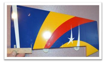
The push-pull control horn is located approximately 9/16" from the bottom of the rudder.
