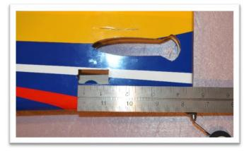
The servo pocket on the <u>right</u> side of the fuselage is used for the rudder servo if you decide to use a push-pull configuration. <u>Do not cut this pocket open if you plan to</u> <u>use the pull-pull cable for the rudder.</u>
