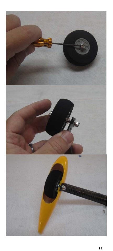
12. Secure the landing gear to the fuselage by inserting a 3mm bolt into a washer, through the carbon fiber gear and into the pre-installed blind nuts in the fuselage. Make sure to use a drop of blue Loctite on each bolt to prevent them from backing out.
