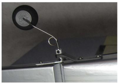
18. Use the hardware provided with the servos to install the rudder and elevator servos in their respective locations in the rear of the aircraft. The rudder and elevator servo linkages assemble and are installed just like the aileron linkages. For maximum control surface travel we highly recommend using the Long Dubro Super Strength servo arms. (Dubro part #670 for Futaba, #671 for JR and #672 for Hitec).
