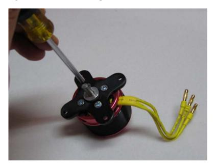
21. Secure the prop adapter using the 4 socket head cap bolts. Again blue Loctite should be applied to each bolt.
