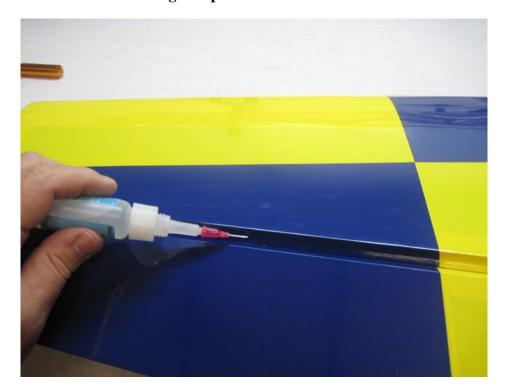
6. Before installing the aileron servo take a minute and <u>apply some CA to the servo tray, root rib and the anti-rotation pins.</u>
