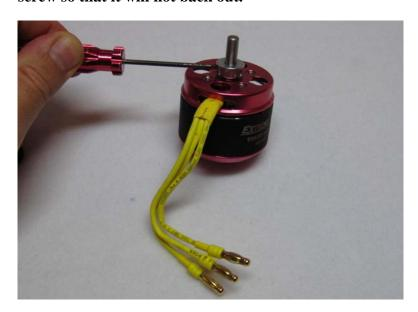
20. Next secure the radial mount to the motor using the provided short Phillip's head machine screws. Again be sure to use a drop of blue Loctite on each screw.
