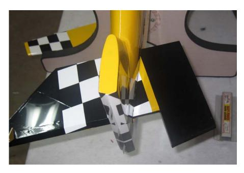
14. Slide the horizontal stabilizer into place. Slide the carbon fiber wing tube into place to use as a reference to ensure that the stab is properly aligned. Use a ruler to make sure the stab is centered in the slot. Sand or shim the slot as necessary to make sure the stab is parallel to the wing tube. Once satisfied glue the stab in place with CA.
