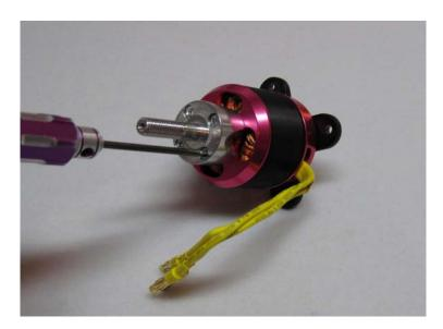
22. Mount the Torque motor using the supplied 4mm black socket head cap bolts and washers. The bolts are to be inserted into the blind nuts which are pre-installed in the motor mount plate. Be sure to put a drop of blue Loctite onto each bolt to prevent them from backing out. Be sure to add some CA to all motor box joints!
