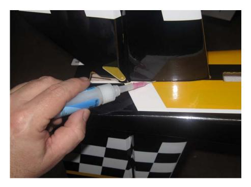
15. Slide the elevator onto the hinges in the stabilizer and secure with thin CA. Again a fresh bottle of CA and a fine glue tip work best here.
