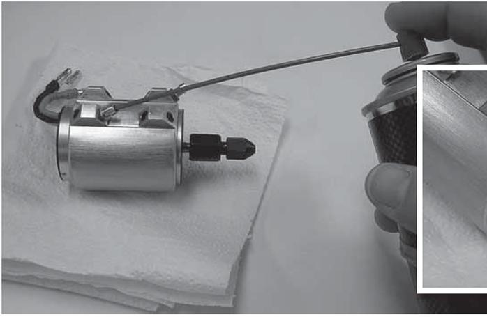
Place the motor in a rag or paper towel and spray a water displacer into the fittings on the water jacket as well as in the motor itself. After the motor is “pickled,” re-oil the motor bearings, wipe the motor down and reinstall it in the boat using the above instructions in reverse order.
