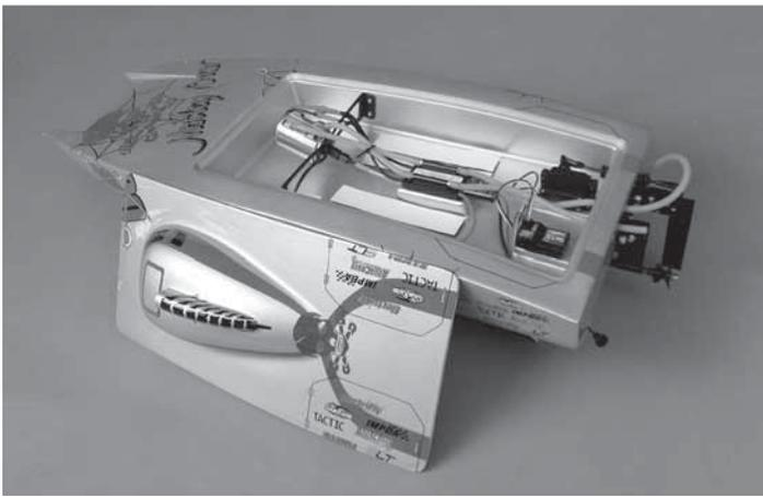
At the end of the day make sure to leave the cowl off and the drain plug out overnight. This will allow any moisture that collected in the boat to safely evaporate.
