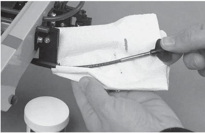
After each 5 or so runs and/or after a day of running it's a good idea to re-lubricate the drive cable. Loosen the cable coupler using the 10 and 12 mm wrenches. Firmly pull the prop and drive shaft out of the back of the boat. Wipe away any old grease and water. Apply new speed grease to the shaft and slide it back into the strut, moving it in and out as you do so to help spread the grease along the length of the cable.
