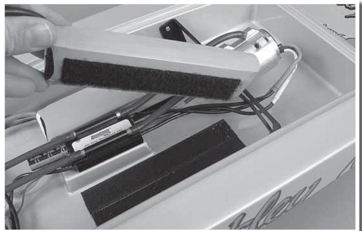
Install the batteries, making sure they are well seated.
