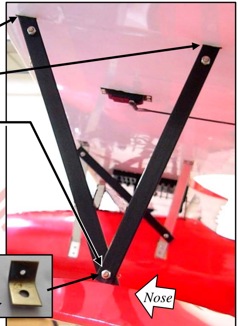
Position the wing-wire anchors toward the fuselage on the 5/8-inch (15mm) bolts (NOTE: Hardware may vary.)
