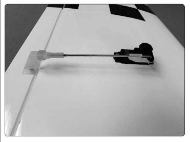
□ 9. Make a 90 degree bend at the mark on each pushrod and cut off the excess pushrod 1/4" [6mm] beyond the bends. Attach the pushrods to the servo arms using nylon FasLinks. Thread the clevises in or out on the pushrods as necessary to center the ailerons with the servo arms still perpendicular to the servo cases. (Never center the servo with the power on.) When satisfied, slide silicone clevis retainers onto the ends of the clevises to secure them.
