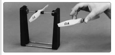
Carefully balance your propeller and spare propellers before you fly. An unbalanced prop can be the single most significant cause of vibration that can damage your model. Not only will motor mounting screws loosen, possibly with disastrous effect, but vibration may also damage your radio receiver and battery.
