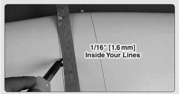
Use a straightedge to guide the soldering iron at a rate that will just melt the covering and not burn into the wood. The hotter the soldering iron, the faster it must travel to melt a fine cut. Peel off the covering.
