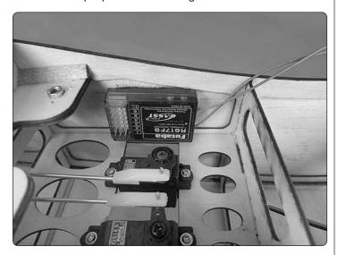
☐ 11. When the epoxy from the previous step has completely cured, use a piece of the included self-adhesive hook and loop material to attach the receiver as shown.
