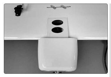
☐ 18. Use a sharp hobby knife to trim the covering from two of the elliptical cutouts in the bottom of the nacelle frames. This will allow cool air to pass over the motors and ESCs and then exit the nacelle frames.
