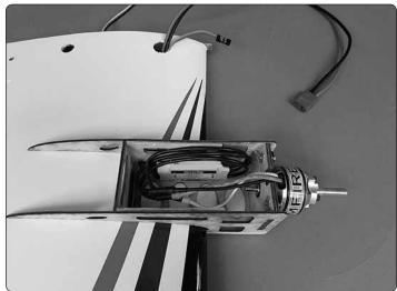
☐ 14. Connect an ESC to the battery Y-harness end you inserted through the wing. Use one of the included tie straps to secure the connectors together as shown. Use a piece of the included double-sided foam tape to stick the ESC to the inside of the nacelle frame where you applied the epoxy coating.
