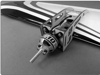
$\Box$  12. Mount the motors to the nacelle firewalls using  $3 \times 12$  mm machine screws, 3mm flat washers, and thread locking compound. Be sure that the motor leads are towards the top of the wing.
