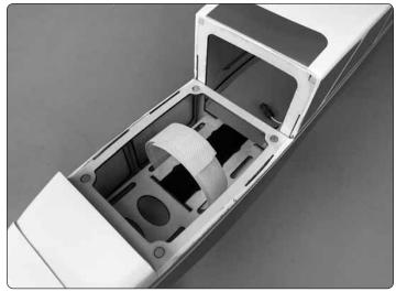
□ 14. Cut a length of non-adhesive hook and loop material 5" [127mm]. Overlap the mating ends approximately 1" [25mm] to make a strap. Put a piece of hook material from the selfahesive hook and loop material and stick it to the battery tray. Fish the strap you made through the middle slots in the battery tray.
