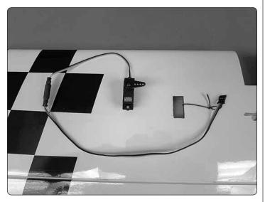
☐ 2. Tie the string ends that are taped inside the wings at the aileron servo bays to the servo extension connectors.
