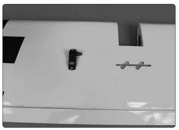
□ 4. Fit the servos into the servo openings and drill 1/16" [1.6mm] holes through the mounting tabs on the servo cases into the rails. Thread a servo mounting screw (included with the servo) into each hole and remove it. Apply a drop of thin CA to each hole to harden the surrounding wood. When the CA has hardened, install the servos into the openings as shown using the screws supplied with the servos.
