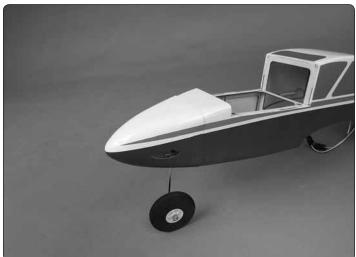
□ 13. Mark the location of the nose gear wire onto the nose cone when you hold it up in place. Use a rotary tool to cut a slot for the wire. The nose cone can be glued, screwed (screws not included) or taped on. We prefer using tape on this model because it allows easy access to the nose gear as well as looking better. If you decide to glue it on then we recommend RTV silicone.
