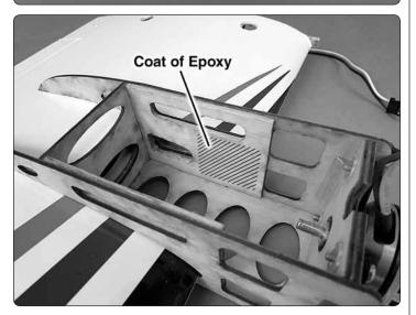
□ 10. Locate the plywood nacelle frames. Coat the wing pockets and aft ends with epoxy and fit the frames into the cutouts in the wings. Wipe away any excess epoxy with a paper towel wetted with denatured alcohol. Use tape to hold them in place. With epoxy still wet, put a thin coating on the inside wall in the location shown on each frame. This will provide a smooth surface to mount the ESC.
