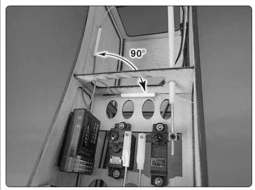
□ 12. Cut the included 4"[100 mm] length of white tube into two equal pieces. Use CA to glue the pieces 90 degrees to each other near the receiver. Feed the antenna wires into the tubes. Note: some receivers may have only one antenna or no exposed antennas at all. Consult your radio manual for requirements for positioning the antenna(s).
