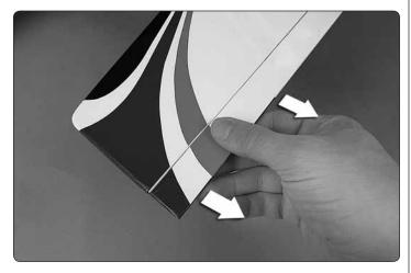
□ 1. Grasp each control surface at one end, taking care not to dent or puncture the covering or the wood structure beneath. Pull the control surface away from the hinge line. Move your hand along the surface and repeat the check for the entire length of the surface.
