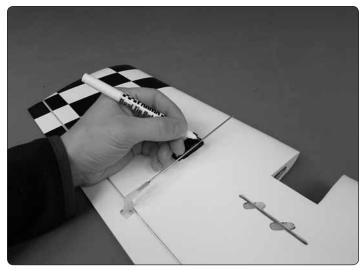
□ 8. With the ailerons in the neutral position (use tape or small clamps to hold them in place), mark the pushrod wires where they cross the enlarged holes in the servo arms.
