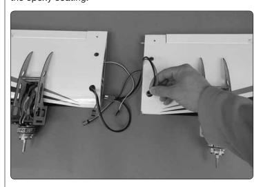
☐ 15. Feed the other female end of the battery Y-harness through the wing sheeting hole in the other wing panel and into the nacelle frame. Connect the ESC to the battery
