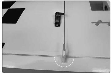
☐ 6. Separate the back plates from two control horns using a knife or sprue cutters. Connect the clevises on the aileron
