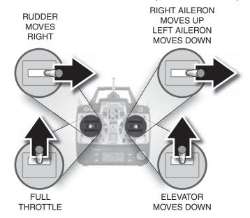
□ 4. Make certain that the control surfaces and the throttle respond in the correct direction as shown in the diagram. If any of the controls respond in the wrong direction, use the servo reversing in the transmitter to reverse the servos connected to those controls. Be certain the control surfaces have remained centered. Adjust if necessary.
