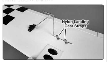
□ 19. Fit the main landing gear wires into the slots in the wing. Place nylon landing gear straps into the cutouts in order to mark the locations for the screw holes. Drill 5/64" [2 mm] holes at the marks you made. Thread a #4 x 3/8" [9.5 mm] washer head screw into each hole and then remove it. Apply a drop or two of thin CA to each hole to harden the surrounding wood. Let the glue harden without accelerator. Install the straps in place using four washer head screws. Repeat for the other side.
