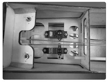
□ 8. Install the rudder and elevator servos onto the tail servo tray using the hardware included with the servos. Use the position of the tail pushrods as they exit the pushrod tubes to determine the location of the servos on the tray. The servos should be aligned so that the pushrods overlap the enlarged holes in the servo arms. Be sure to harden the wood surrounding the mounting screw holes with thin CA. Center the servos with the radio.
