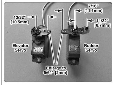
Install servo arms onto the elevator and rudder servos as shown. A brass screw lock connector is needed for the nose gear pushrod. Enlarge the holes for the rudder and elavator pushrods using a 5/64" [2 mm] drill bit. We chose a high torque servo for the rudder for more responsive yaw control in flight.
