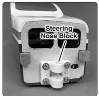
☐ 1. Mount the steering nose block onto the front of the fuselage using four 3x12mm machine screws, four 3mm flat washers and thread locking compound.
