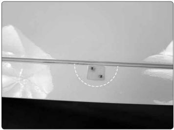
☐ 7. Use a felt-tip pen to mark the location of the control horn mounting holes onto both ailerons.
