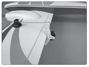
Use a Great Planes AccuThrow (or a ruler) to accurately measure and set the control throw of each control surface as indicated in the chart that follows. If your radio does not have dual rates, we recommend setting the throws at the **low** rate setting.
