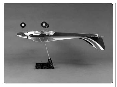
☐ 2. With the wing attached to the fuselage and all parts of the model installed (ready to fly), place the model on a Great Planes CG Machine upside down, or lift it at the balance point you marked.
