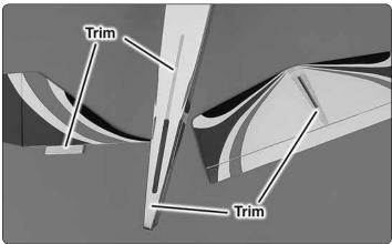
□ 4. Fit the vertical fin and horizontal stabilizer into place. Use a felt tip marker to trace around the fuselage onto the tail parts top and bottom and left and right side. Trace around the fin onto the fuse. Remove the tail parts and trim the covering away 1/16" [1.6mm] inside your lines as shown.
