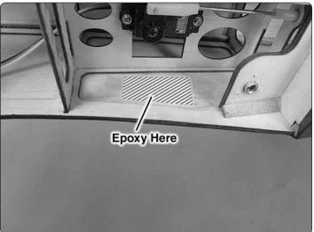
□ 10. Mix up a small batch of epoxy and apply a thin coat to the battery tray and the side of the fuselage by the elevator servo for the purpose of attaching the receiver.
