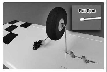
□ 20. Slide a 3.5mm wheel collar followed by the wheel, then another 3.5mm wheel collar. Use a felt tip pen to mark the
