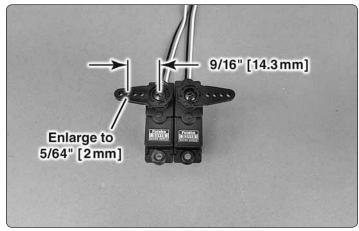
□ 1. Center your aileron servos with your radio system. Test fit four-armed servo arms onto the servos to determine
