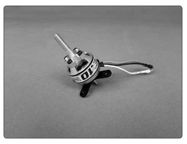
☐ 11. Install the aluminum X-mount onto the motors using the screws included with the motors and thread locking compound. Install the prop adapters using the screws included with the motors and thread locking compound.
