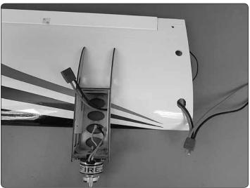
☐ 13. Feed one of the female ends of the battery Y-harness through the forward wing sheeting hole in one wing panel. Manuever it through the wing ribs and into the nacelle frame.
