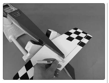
□ 6. Thread a nylon clevis onto a 27" [685 mm] pushrod. Attach the clevis to a control horn and slide the pushrod into the outer pushrod tube on the right side of the fuse. As you did with the ailerons, align the control horn over the elevator hinge line and mark the location of the screw holes. Drill 5/64" [2mm] holes at your marks and install the horn using two 2-56 x 3/8" [9.8 mm] machine screws and the control horn backplate.
