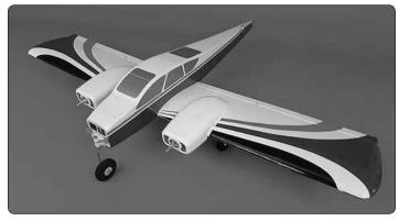
$\square$  3. Temporarily mount the wing to the fuselage using the two 10-24 x 2" [51 mm] nylon wing bolts.
