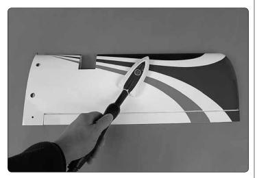
□ 2. Use a covering iron with a covering sock on high heat to tighten the covering if necessary. Apply pressure over sheeted areas to **thoroughly** bond the covering to the wood. Take care when applying heat onto trim covering applied over the base color. Move the iron at a rate slow enough to get the covering hot but not so slow that the top color shrinks on top of the base color causing the edges to pull away.
