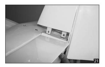
4. Remove the covering from the fuselage.
