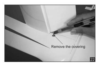
5. Secure the vertical stabilizer into the fuselage.
