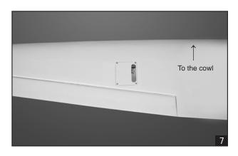
7. Using masking tape, tape the servo leads on to the top of the wing.
